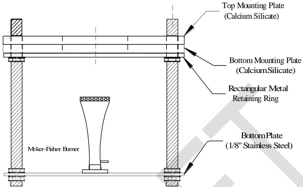
Side view of the horizontal test apparatus
