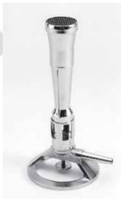
Figure B-1. Meker-Fisher Gas Burner
