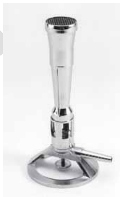
Figure B-1. Meker-Fisher Gas Burner
